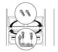
7. Unscrew the retaining screw for the self-closing mechanism on the bottom of the fridge compartment door.
